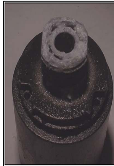
POWDER COAT MASKING, 0.005" THICK
